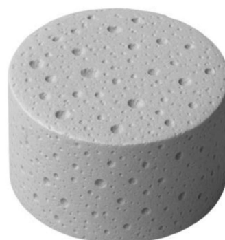
Figure 4. Porous structure of tablet formed by sublimation system 37
