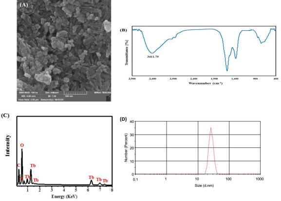
Figure 1. (A) SEM image; (B) FT-IR spectrum; (C) EDX (D) DLS of the DMF-Tb-Phen MOF NPs.
