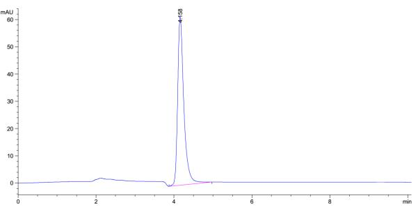
Figure 2. Chromatogram of 5 µg/mL acrylamide spiked in chips sample and analyzed using US-LLE/HPLC-UV.
