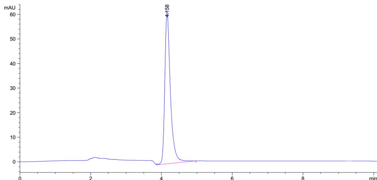
Figure 2. Chromatogram of 5 µg/mL acrylamide spiked in chips sample and analyzed using US-LLE/HPLC-UV.
