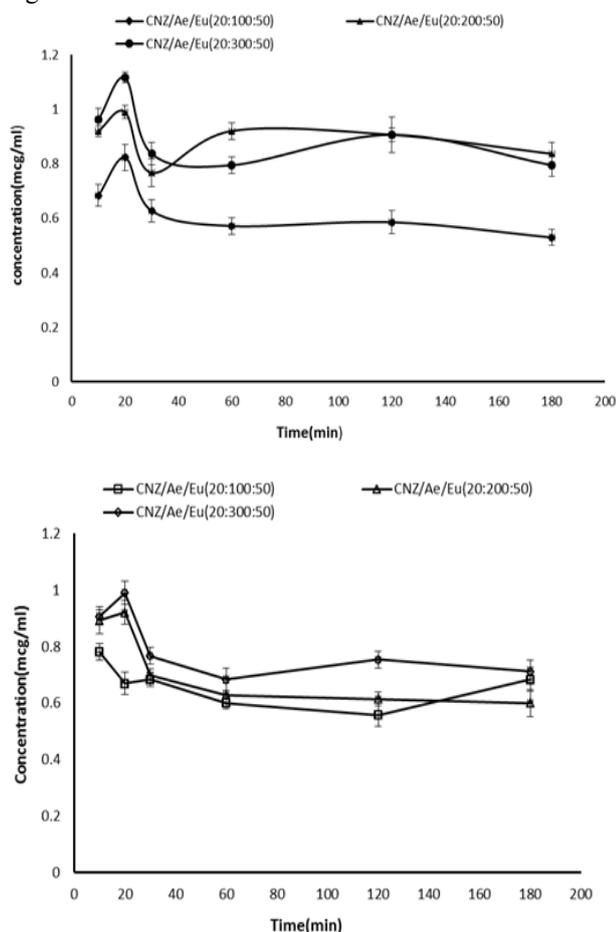
**Figure 6.** In vitro release of up: CNZ loaded Ae blended with Eu at different CNZ/Ae ratios and down: CNZ-Eu co-loaded Ae at different CNZ/Ae ratios.
