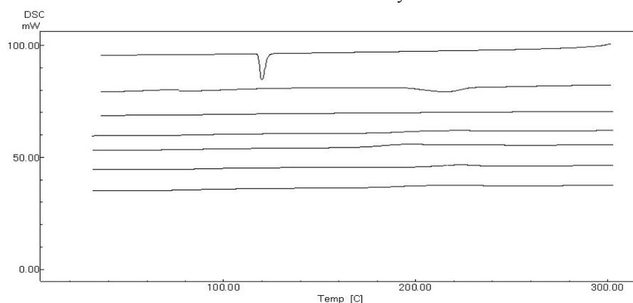
**Figure 2.** DSC scans of the samples from up to down: plain CNZ, Eu, Ae, CNZ loaded Ae (1:5), CNZ loaded Ae (1:15), CNZ-Eu coloaded Ae (1:5:2.5) and CNZ loaded Ae (1:5) after 3 month.
