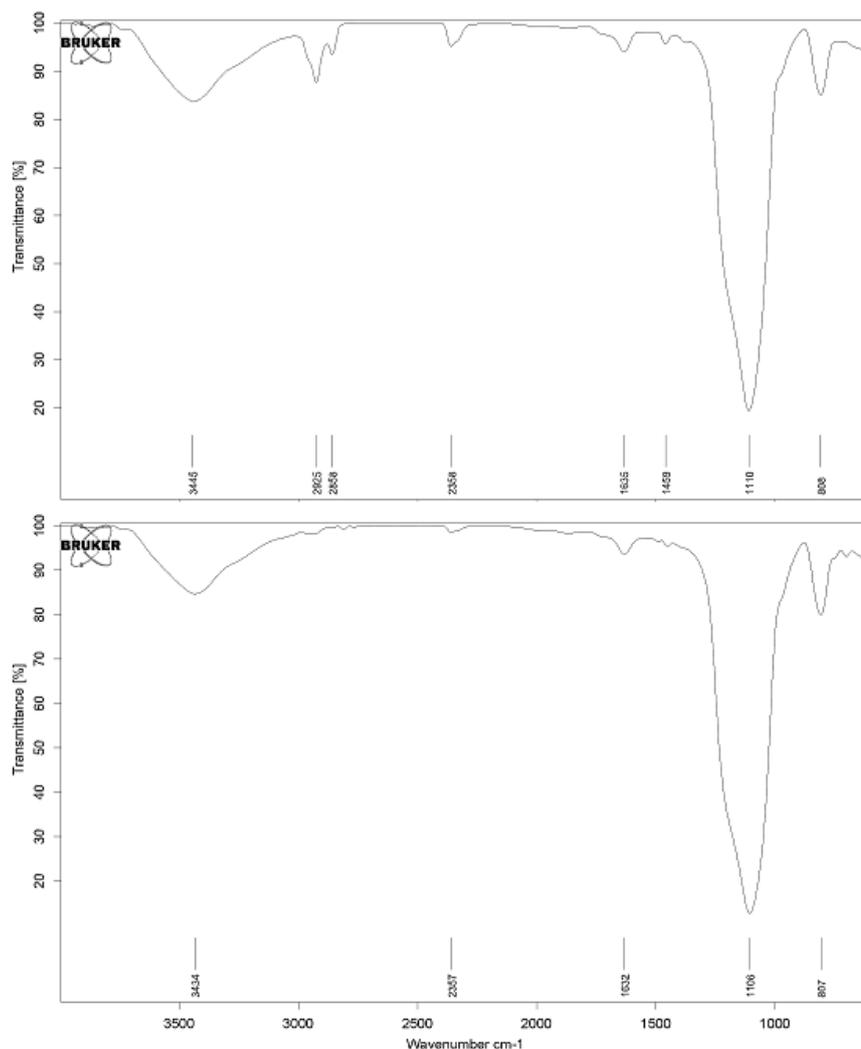
**Figure 3.** FT-IR of spectrum of samples (up) Ae, (down) CNZ loaded Ae.
