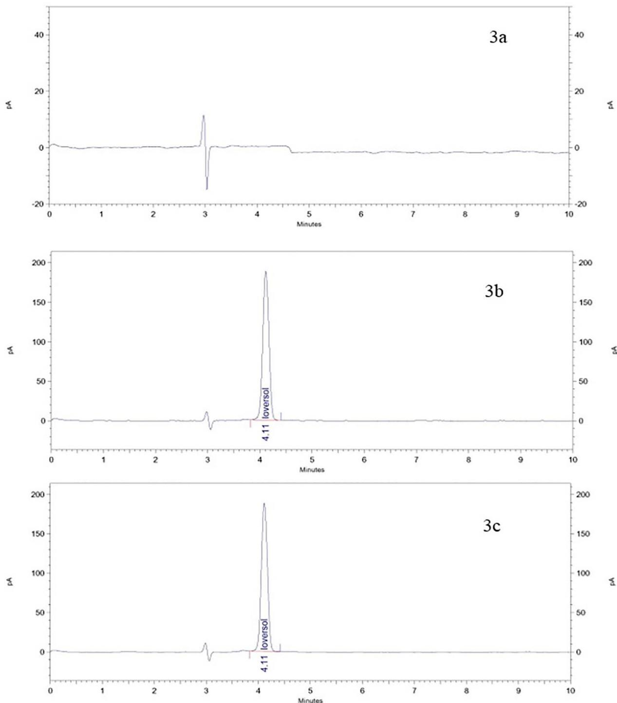
**Figure 3.** Chromatogram of (a) Mobile phase blank (b) IVL standard solution,  $R_t = 4.11$  min (c) IVL injection sample solution,  $R_t = 4.11$  min.
