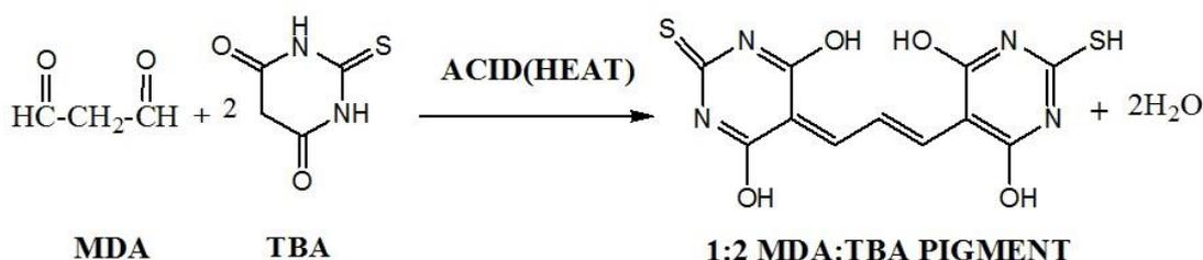
Figure 1. Schematic representation of reaction between TBA and MDA.
