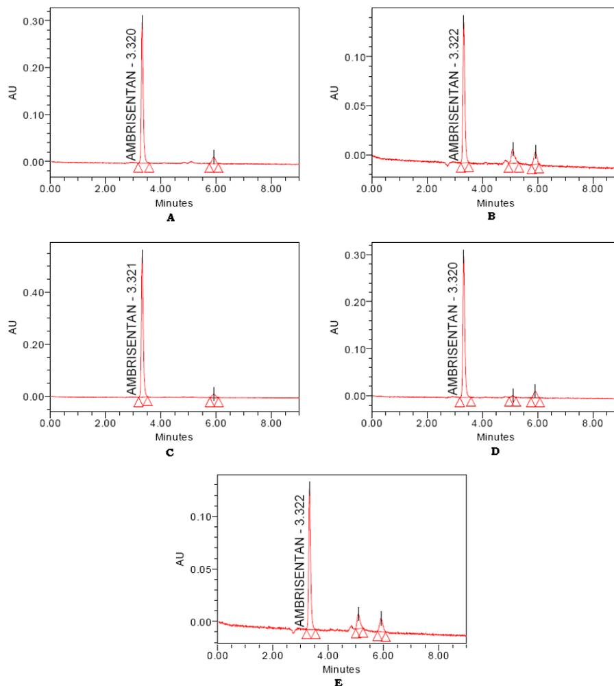
**Figure 2.** Chromatograms of the samples that have subjected to (A) Acid hydrolysis (B) Alkali hydrolysis (C) Oxidative stress (D) Dry heat (E) Sun Light
