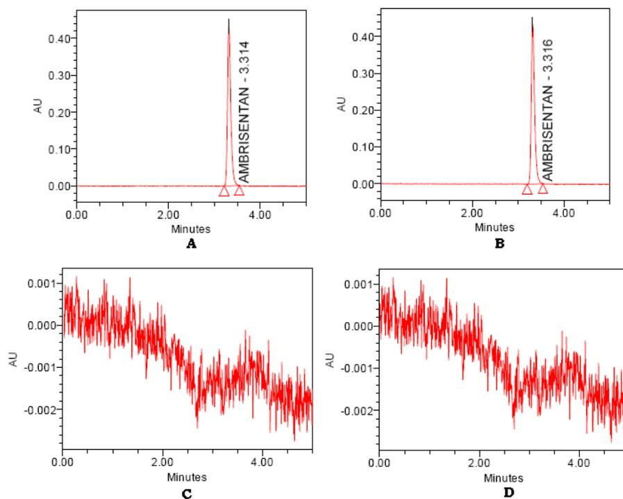
**Figure 1.** Chromatogram of (A) Pure sample (B) Tablet sample (C) Placebo (D) Blank mobile phase
