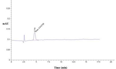
Figure 1. The chromatogram of mixed standard solution of oxytetracycline (100 ng/g).
